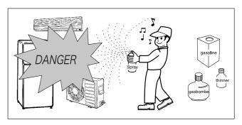
13. If refrigerant gas leaks, be sure to repair the leak(s) securely before recharge the unit. Refrigerant (R32) is harmless. However when comes in contact with fire will generate toxic gas.
